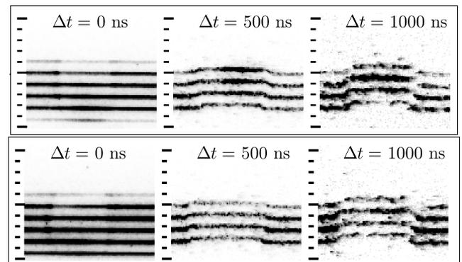
Fig. 4. Single-shot fluorescence exposures for  $95\% \text{ air}/5\% \text{ Kr}$  jet experiments with laser diode (top) and single-laser scheme (bottom). Tick marks are  $1 \text{ mm}$ . Flow is bottom to top. Inverted intensity scale.
