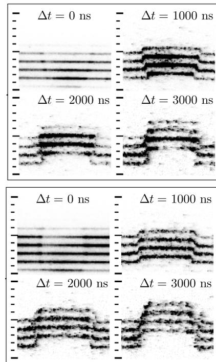
Fig. 3. Single-shot fluorescence exposures for  $99\% \text{ N}_2/1\% \text{ Kr}$  jet experiments with laser diode (top four) and single-laser scheme (bottom four). Tick marks are  $1 \text{ mm}$ . Flow is bottom to top. Inverted intensity scale.
