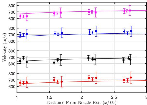
**Fig. 6.** Measured underexpanded jet velocity. Legend in Fig. 5. Error bars represent uncertainty estimate. Write/read delay times are denoted by circle, square, triangle, diamond, and  $x$  for 500, 1000, 1500, 2000, and 3000 ns, respectively.
