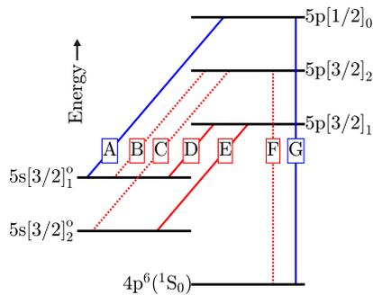
**Fig. 1.** Energy diagram. Racah  $n[K]_j$  notation. Scheme marked in red utilizes conventional 214.7 nm excitation with re-excitation by laser diode at 769.7 nm. Scheme marked in blue uses excitation at 212.56 nm with successive camera gating (no read laser). Transition details in Table 1.
