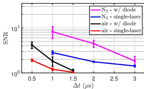
**Fig. 5.** Mean SNR versus delay for underexpanded jet experiments. Error bars represent the standard deviation of SNR.
